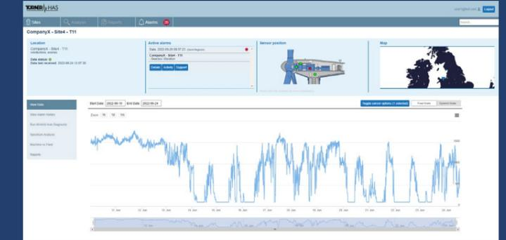
Live data can be viewed as it becomes available every 5 minutes. Multiple parameters can be viewed at any one time in addition to WindSync parameters such as power output or wind speed. Dynamic scaling of the y-axis allows for the relationship between the measured parameter and turbine operating state to be quickly visualised. The data displayed is defaulted to one month but any period of collected data can be viewed by altering the date range.
